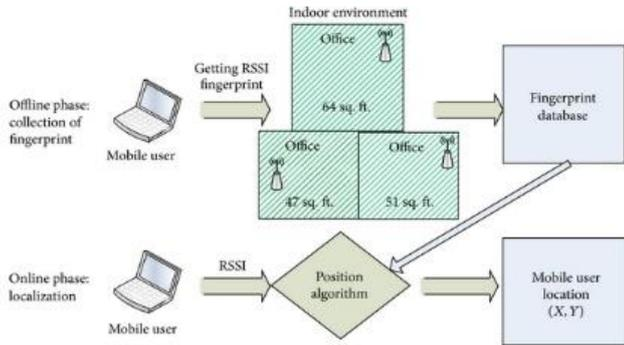
Figure 2: Fingerprinting based Positioning
