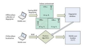
Figure 2: Fingerprinting based Positioning
